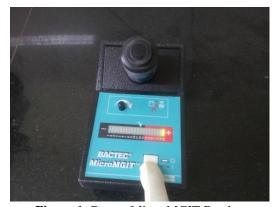
Figure 1: Bactec Micro MGIT Reader.
